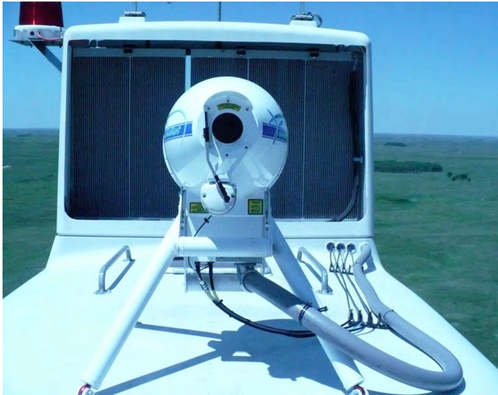
Figure 1 Vindicator ® LWS Installed on T22
